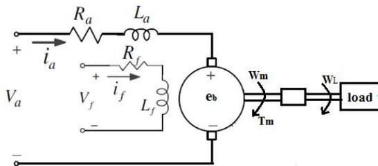
Figure 2: Equivalent circuit of DC motor
