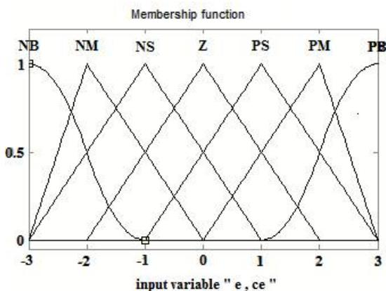
Figure 3: Membership functions of inputs e and ce.
