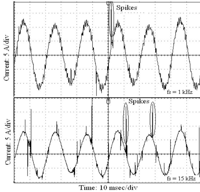
Figure 3: PWM current waveform
