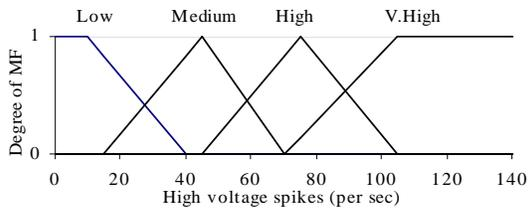
Figure 10: Membership function for high voltage spikes/sec
