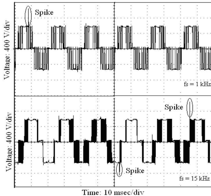
Figure 2: PWM voltage waveform
