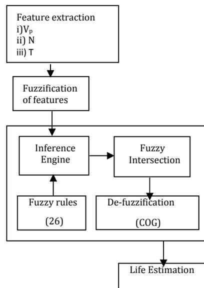
Figure 13: Schematic diagram for flow of information in fuzzy system
