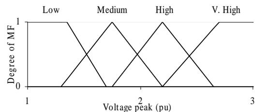
Figure 9: Membership function for voltage peak
