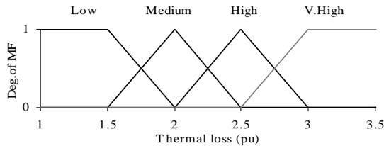
Figure 11: Membership function for thermal loss
